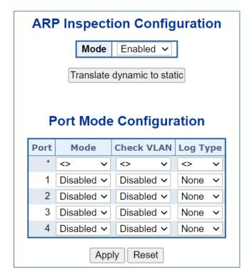
Figure 4-5-32: ARP Inspection Configuration Screen Page Screenshot
