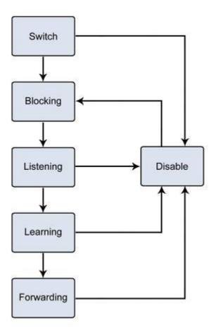
Figure 4-3-35: STP Port State Transitions
