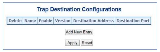
Figure 4-2-23: SNMP Trap Destination Configuration Page Screenshot
