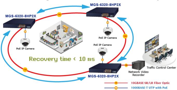
Figure 4-6-2: Ring Example Diagram
