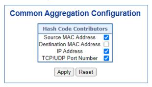
Figure 4-3-12: Common Aggregation Configuration Page Screenshot
