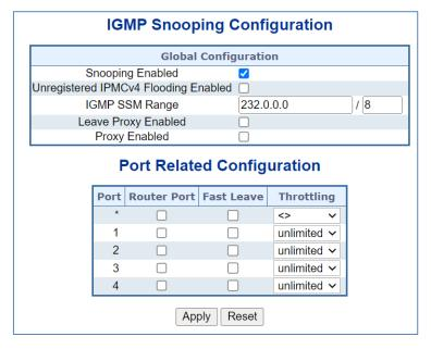
Figure 4-3-49: IGMP Snooping Configuration Page Screenshot
