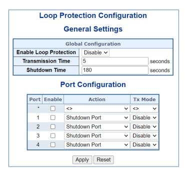
Figure 4-3-72: Loop Protection Configuration Page Screenshot
