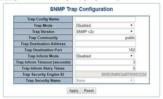
Figure 4-2-24: SNMP Trap Configuration Page Screenshot
