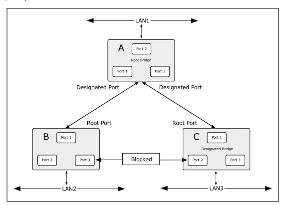
Figure 4-3-37: After Applying the STA Rules
