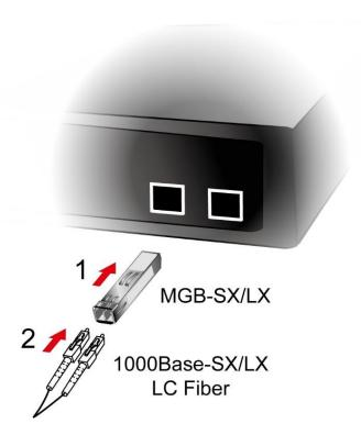
Figure 2-3-1: Plug in the SFP/SFP+ Transceiver
