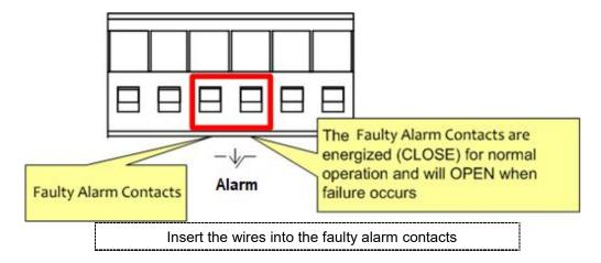
Figure 2-1-8: Fault Alarm Contact for Industrial Managed TSN Device
