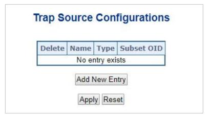
Figure 4-2-25: SNMP Trap Source Configuration Page Screenshot
