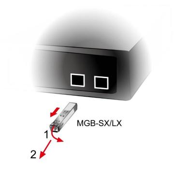
Figure 2-3-2: Pull out the SFP Transceiver Module
