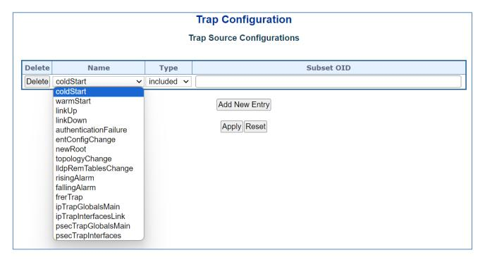
Figure 4-2-26: SNMP Trap Source Configuration Page Screenshot
