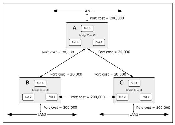
Figure 4-3-36: Before Applying the STA Rules
