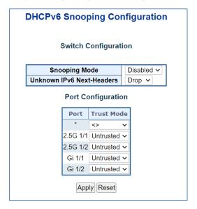
Figure 4-5-25: DHCPv6 Snooping Table Configuration Screen Page Screenshot
