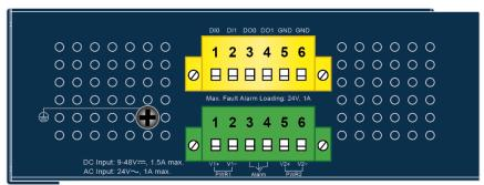
Figure 2-1-5: Industrial Managed TSN Device Upper Panel
